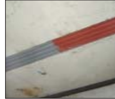
Bottom view (fire side) of intumescent-only and intumescent plus silicone bellows coating.
