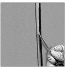
Tool away the excess joining sealant and blend the join.
