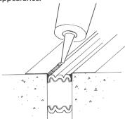
Where TFR-RWS foam meets at butt joins, tool the excess silicone that squeezes out from the top and between the bellows.
