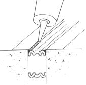
IMPORTANT: Sealant left between the wrinkles of the bellows could constrain movement — using a caulk knife, remove excess sealant and blend what remains into the bellows.
