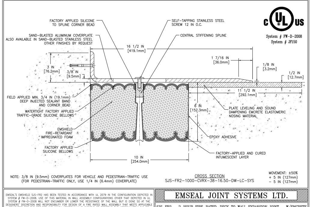
STANDARDS FOR THE PROJECT AND WHICH ADDITIONALLY IS CAPABLE OF RESISTING THE APPROXIMATELY 2.5 PSI (120 LBS PER FOOT OF JOINT BASED ON 4-INCH DEPTH OF SEAL) BACKPRESURE OF THE SJS-FR2 MATERIAL.
