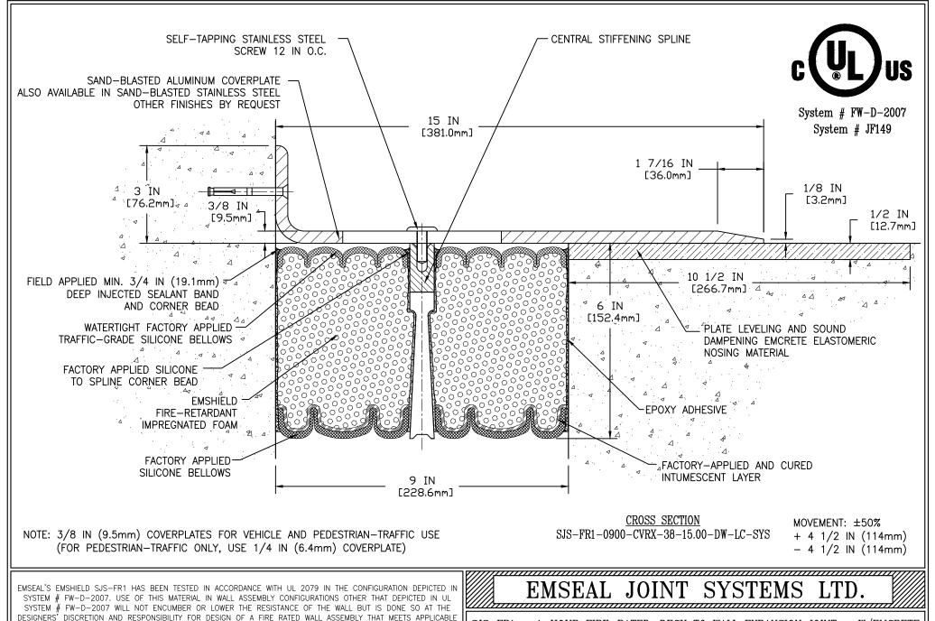
STANDARDS FOR THE PROJECT AND WHICH ADDITIONALLY IS CAPABLE OF RESISTING THE APPROXIMATELY 2.5 PSI (120 LBS PER FOOT OF JOINT BASED ON 4-INCH DEPTH OF SEAL) BACKPRESURE OF THE SJS-FR1 MATERIAL.
