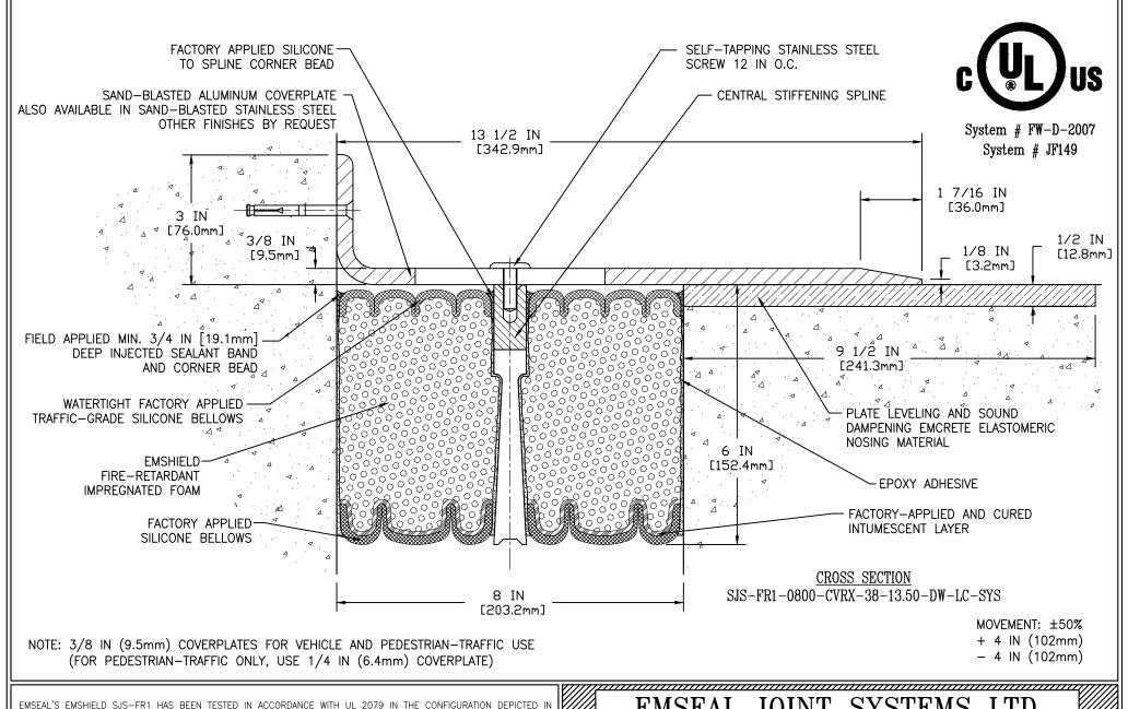
SYSTEM # FW-D-2007. USE OF THIS MATERIAL IN WALL ASSEMBLY CONFIGURATIONS OTHER THAT DEPICTED IN UL SYSTEM # FW-D-2007 WILL NOT ENCUMBER OR LOWER THE RESISTANCE OF THE WALL BUT IS DONE SO AT THE DESIGNERS' DISCRETION AND RESPONSIBILITY FOR DESIGN OF A FIRE RATED WALL ASSEMBLY THAT MEETS APPLICABLE STANDARDS FOR THE PROJECT AND WHICH ADDITIONALLY IS CAPABLE OF RESISTING THE APPROXIMATELY 2.5 PSI (120 LBS PER FOOT OF JOINT BASED ON 4-INCH DEPTH OF SEAL) BACKPRESURE OF THE SJS-FR1 MATERIAL.
