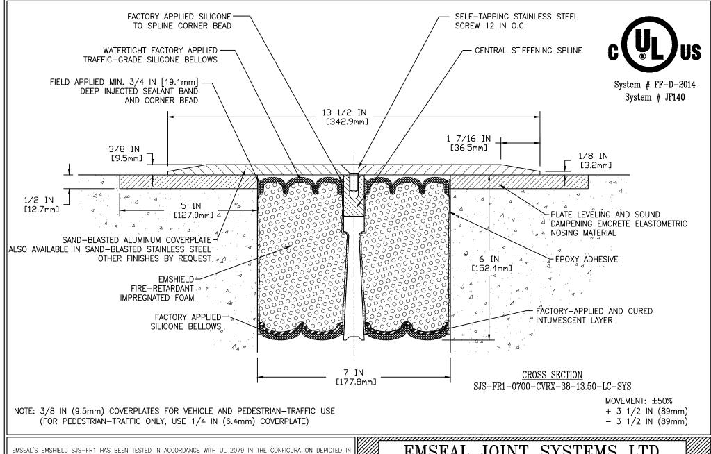
SYSTEM # FF-D-2014. USE OF THIS MATERIAL IN WALL ASSEMBLY CONFIGURATIONS OTHER THAT DEPICTED IN UL SYSTEM # FF-D-2014 WILL NOT ENCUMBER OR LOWER THE RESISTANCE OF THE WALL BUT IS DONE SO AT THE DESIGNERS' DISCRETION AND RESPONSIBILITY FOR DESIGN OF A FIRE RATED WALL ASSEMBLY THAT MEETS APPLICABLE STANDARDS FOR THE PROJECT AND WHICH ADDITIONALLY IS CAPABLE OF RESISTING THE APPROXIMATELY 2.5 PSI (120 LBS PER FOOT OF JOINT BASED ON 4-INCH DEPTH OF SEAL) BACKPRESURE OF THE SJS-FR1 MATERIAL.
