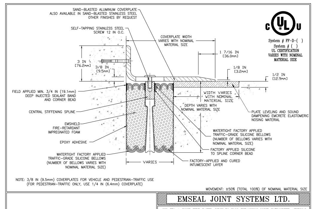
SJS-FR1-1-HOUR FIRE-RATED, DECK TO WALL EXPANSION JOINT-W/EMCRETE- TYPICAL
