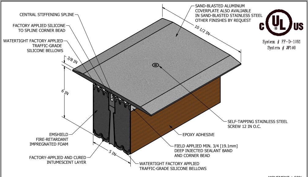
NOTE: 3/8 IN (9.5mm) COVERPLATES FOR VECHILE AND PEDESTRIAN-TRAFFIC USE (FOR PEDESTRIAN-TRAFFIC ONLY, USE 1/4 (6.4mm) COVERPLATE)
