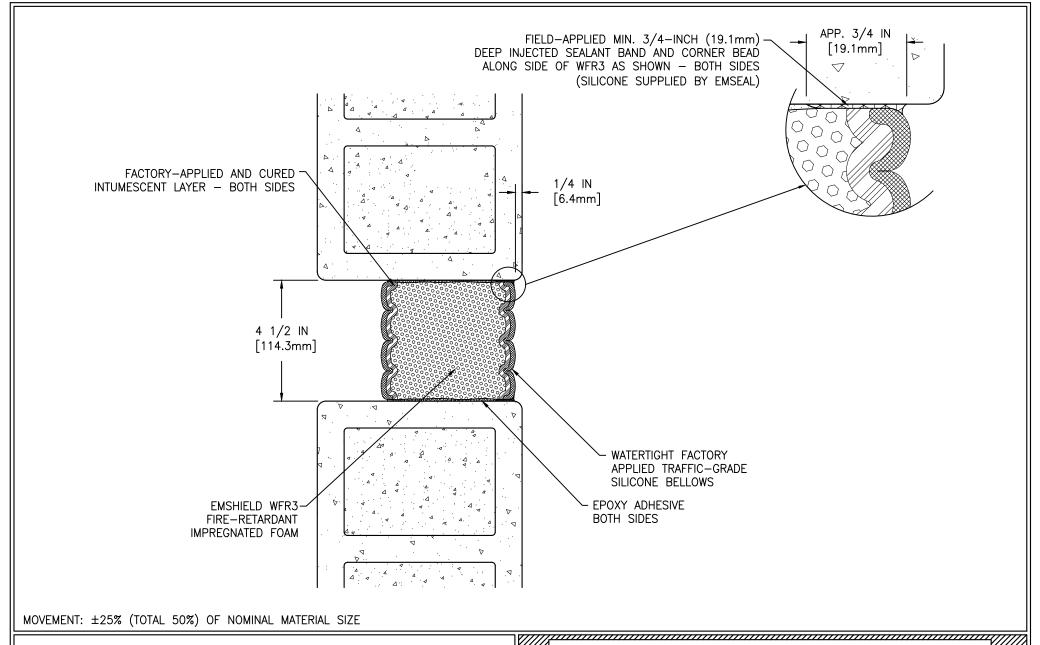
EMSEAL'S EMSHIELD WFR3 HAS BEEN TESTED IN ACCORDANCE WITH UL 2079 IN THE CONFIGURATION DEPICTED IN SYSTEM # WW-D-1087. USE OF THIS MATERIAL IN WALL ASSEMBLY CONFIGURATIONS OTHER THAT DEPICTED IN UL SYSTEM # WW-D-1087 WILL NOT ENCUMBER OR LOWER THE RESISTANCE OF THE WALL BUT IS DONE SO AT THE DESIGNERS' DISCRETION AND RESPONSIBILITY FOR DESIGN OF A FIRE RATED WALL ASSEMBLY THAT MEETS APPLICABLE STANDARDS FOR THE PROJECT AND WHICH ADDITIONALLY IS CAPABLE OF RESISTING THE APPROXIMATELY 2.5 PSI
