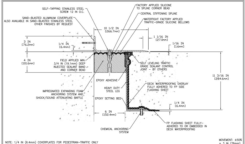
IOTE: 1/4 IN (6.4mm) COVERPLATES FOR PEDESTRIAN—TRAFFIC ONLY (FOR VEHICULAR AND PEDESTRIAN—TRAFFIC, USE 3/8 IN (9.5mm) COVERPLATE)
