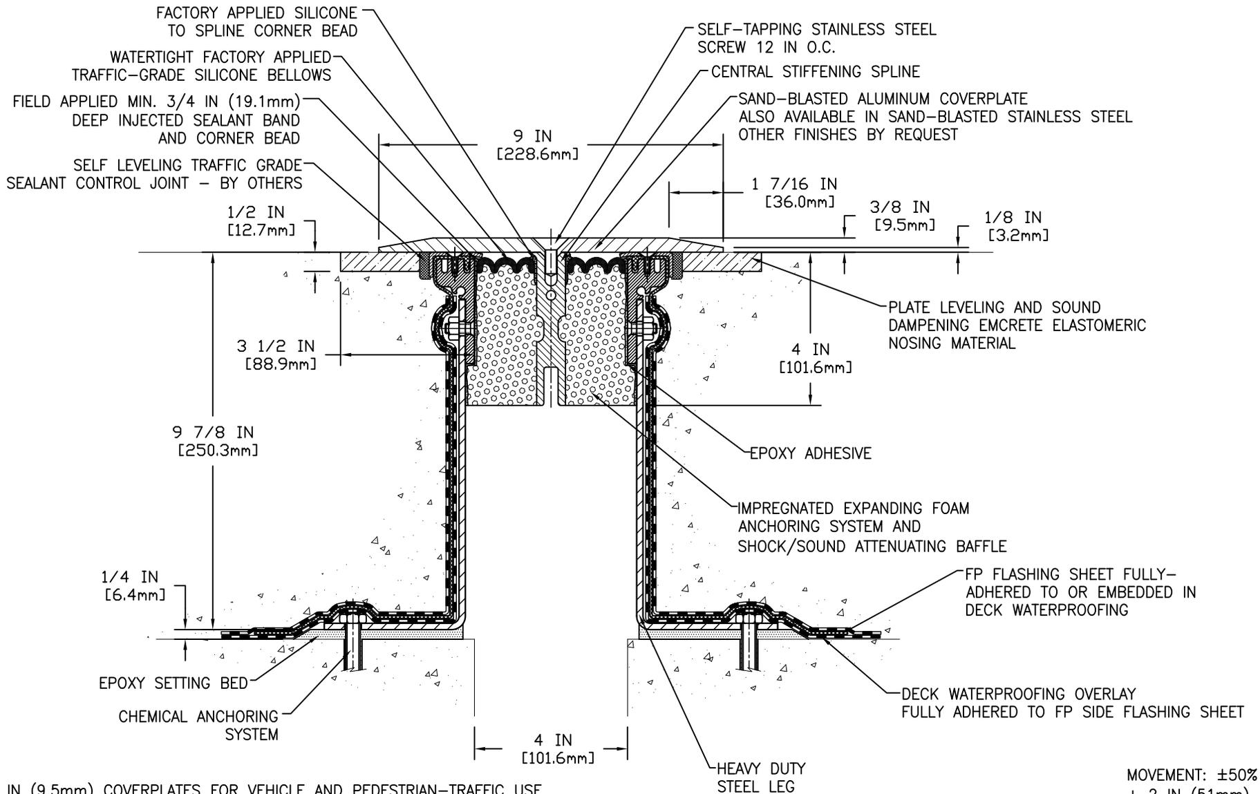
NOTE: 3/8 IN (9.5mm) COVERPLATES FOR VEHICLE AND PEDESTRIAN-TRAFFIC USE
