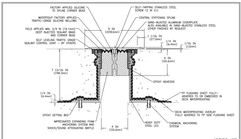
NOTE: 1/4 IN (6.4mm) COVERPLATES FOR PEDESTRIAN—TRAFFIC ONLY (FOR VEHICULAR AND PEDESTRIAN—TRAFFIC, USE 3/8 IN (9.5mm) COVERPLATE)
