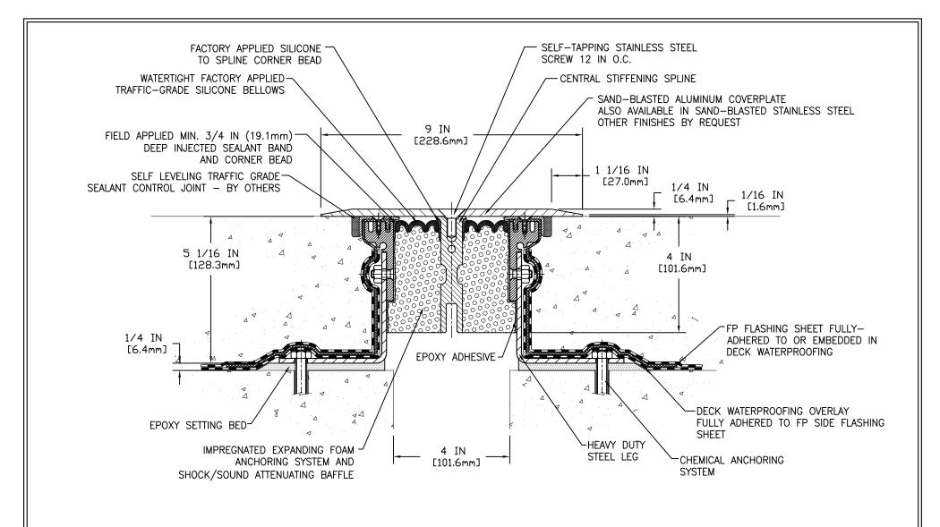
NOTE: 1/4 IN (6.4mm) COVERPLATES FOR PEDESTRIAN—TRAFFIC ONLY (FOR VEHICULAR AND PEDESTRIAN—TRAFFIC, USE 3/8 IN (9.5mm) COVERPLATE)
