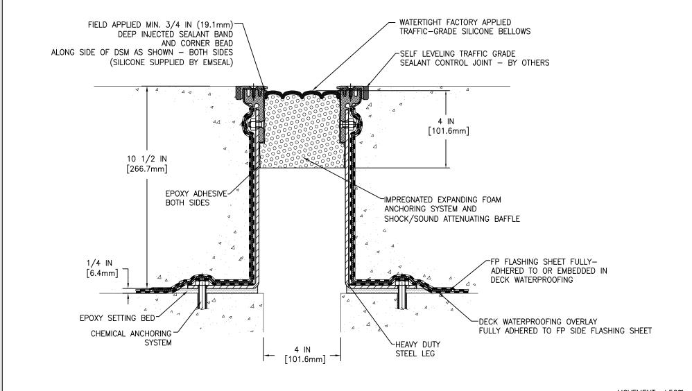
MOVEMENT: ±50% + 2 IN (51mm) - 2 IN (51mm)
