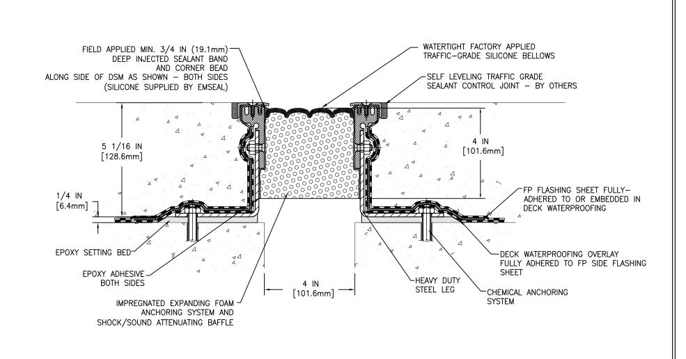
MOVEMENT: ±50% + 2 IN (51mm) - 2 IN (51mm)
