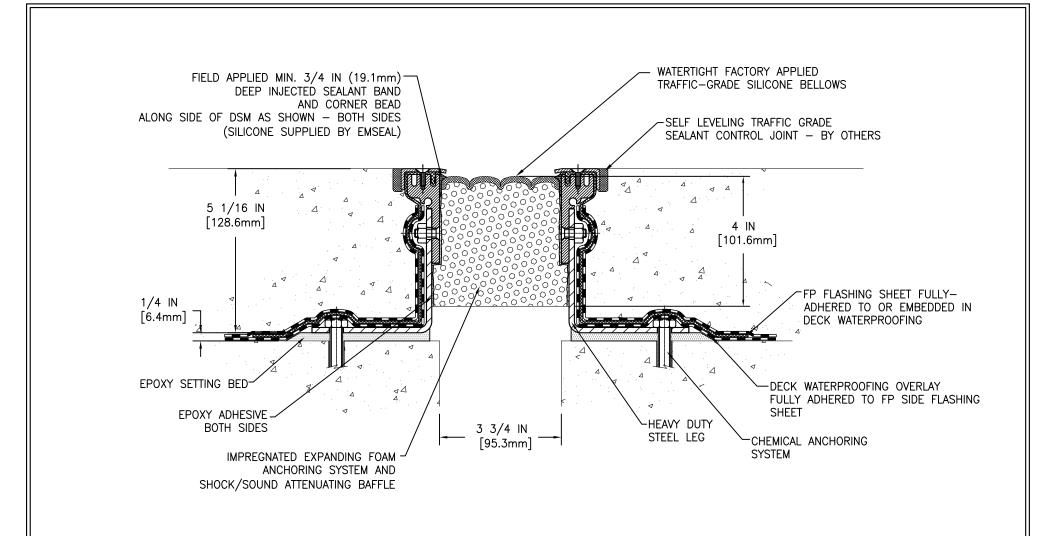
MOVEMENT: ±50% + 1 7/8 IN (48mm) - 1 7/8 IN (48mm)
