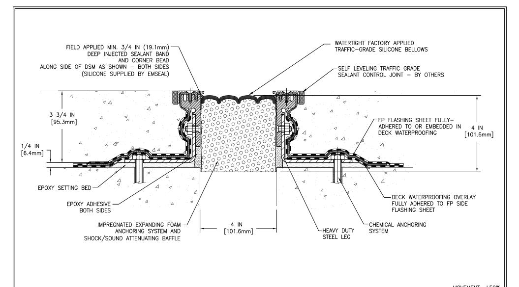
MOVEMENT: ±50% + 2 IN (51mm) - 2 IN (51mm)
