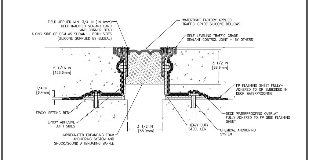
MOVEMENT: ±50% + 1 3/4 IN (45mm) - 1 3/4 IN (45mm)
