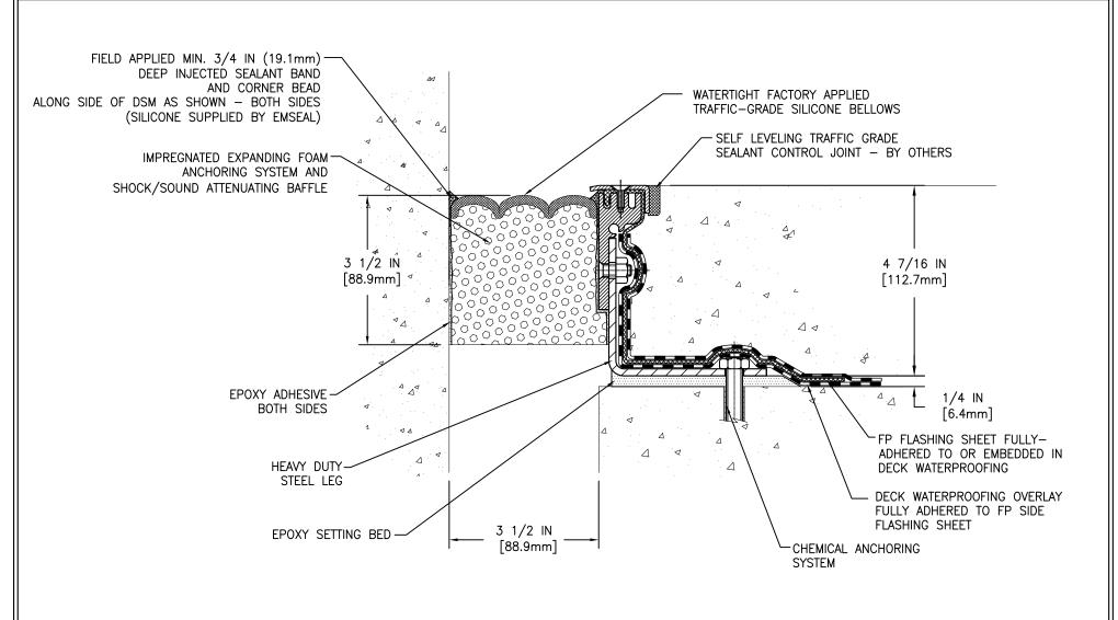
MOVEMENT: ±50% + 1 3/4 IN (45mm) - 1 3/4 IN (45mm)
