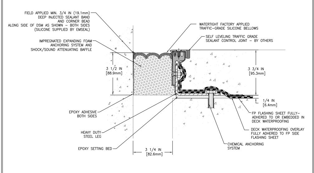
MOVEMENT: ±50% + 1 5/8 IN (41mm) - 1 5/8 IN (41mm)
