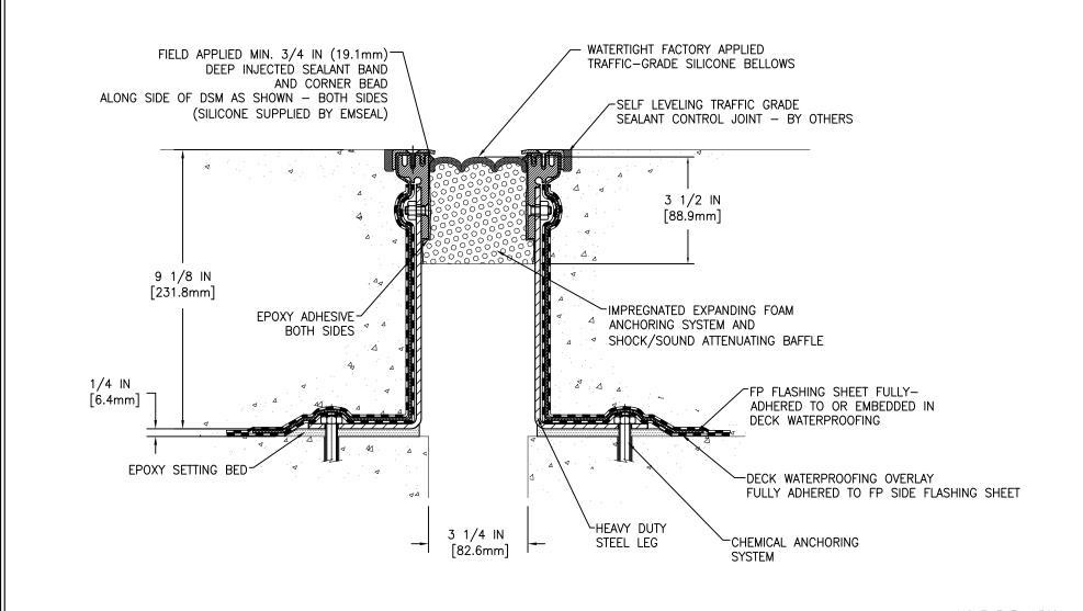
MOVEMENT: ±50% + 1 5/8 IN (41mm) - 1 5/8 IN (41mm)
