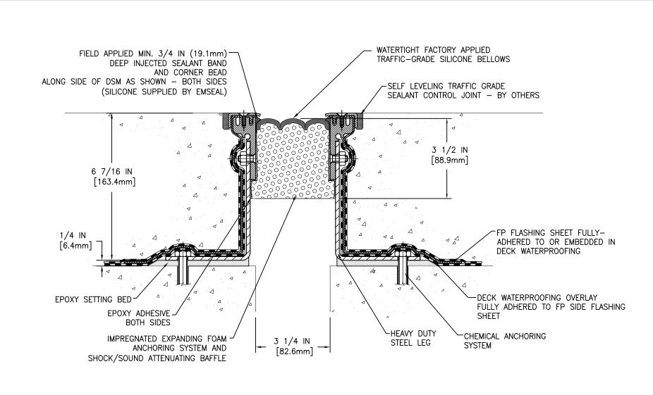
MOVEMENT: ±50% + 1 5/8 IN (41mm) - 1 5/8 IN (41mm)
