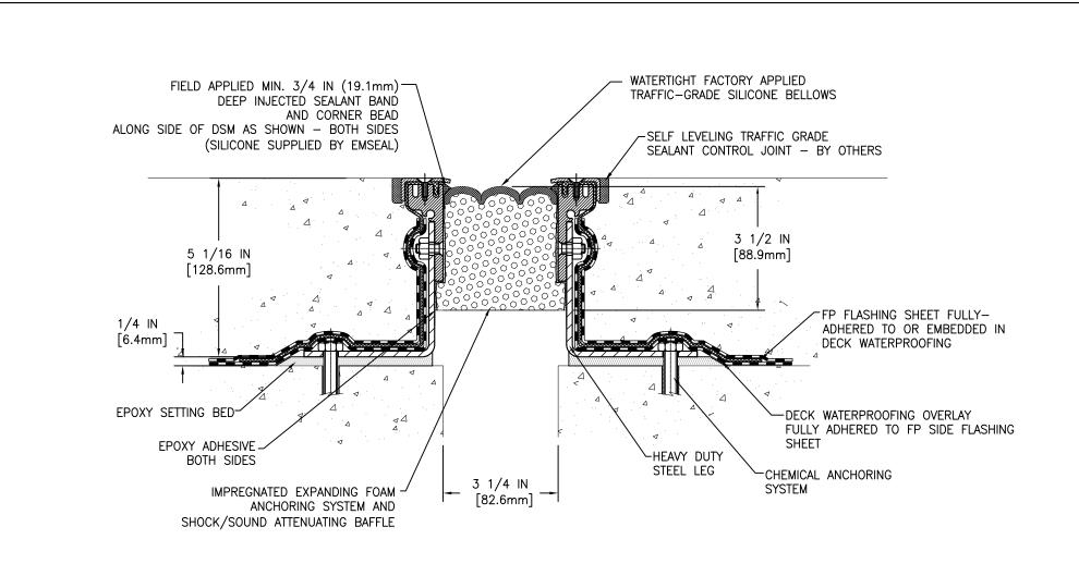
MOVEMENT: ±50% + 1 5/8 IN (41mm) - 1 5/8 IN (41mm)
