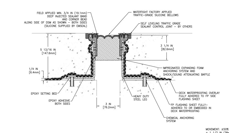
MOVEMENT: ±50% + 1 1/2 IN (38mm) - 1 1/2 IN (38mm)
