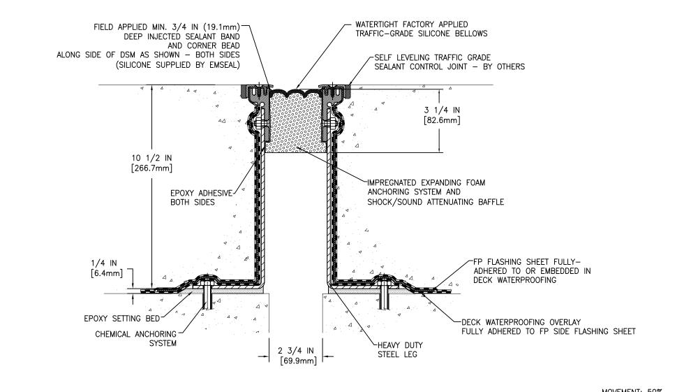
MOVEMENT: 50% + 1 3/8 IN (35mm) - 1 3/8 IN (35mm)
