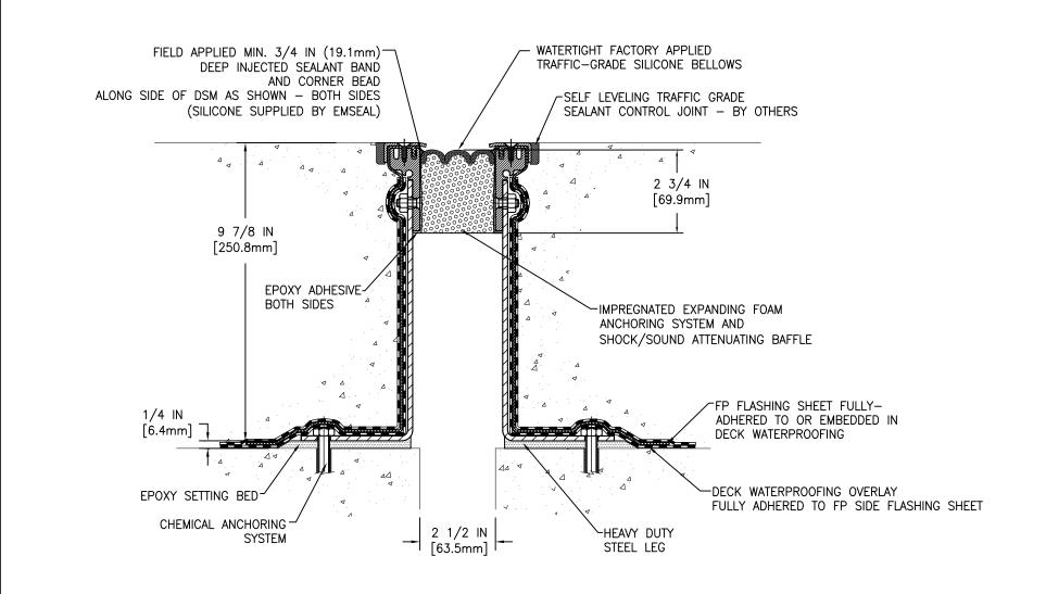
MOVEMENT: ±50% + 1 1/4 IN (32mm) - 1 1/4 IN (32mm)
