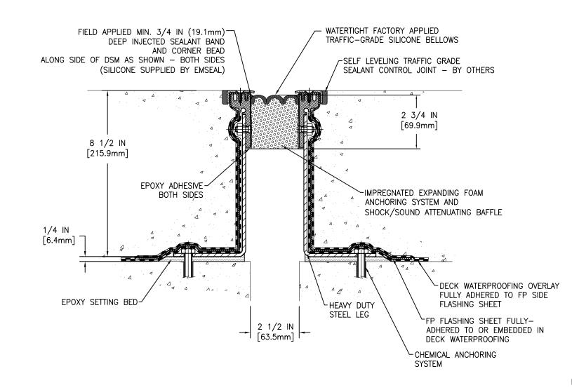
MOVEMENT: ±50% + 1 1/4 IN (32mm) - 1 1/4 IN (32mm)
