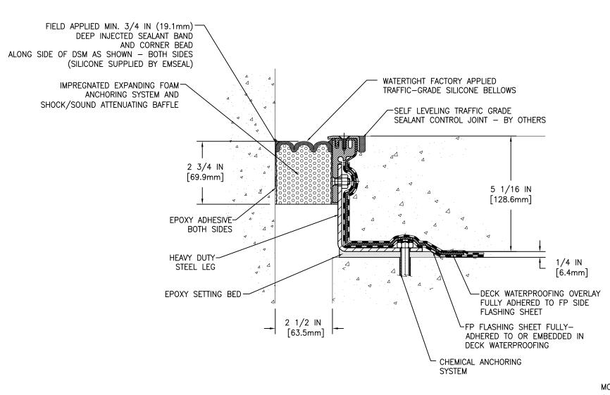
MOVEMENT: ±50% + 1 1/4 IN (32mm) - 1 1/4 IN (32mm)
