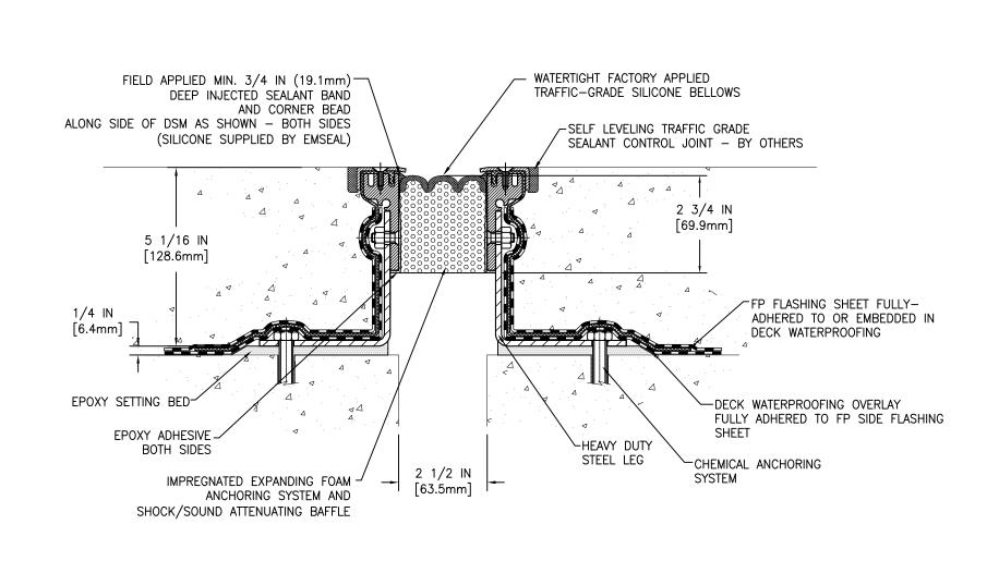
MOVEMENT: ±50% + 1 1/4 IN (32mm) - 1 1/4 IN (32mm)
