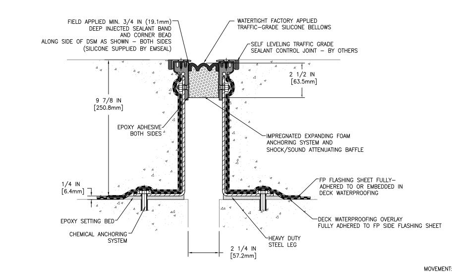
MOVEMENT: ±50% + 1 1/8 IN (29mm) - 1 1/8 IN (29mm)
