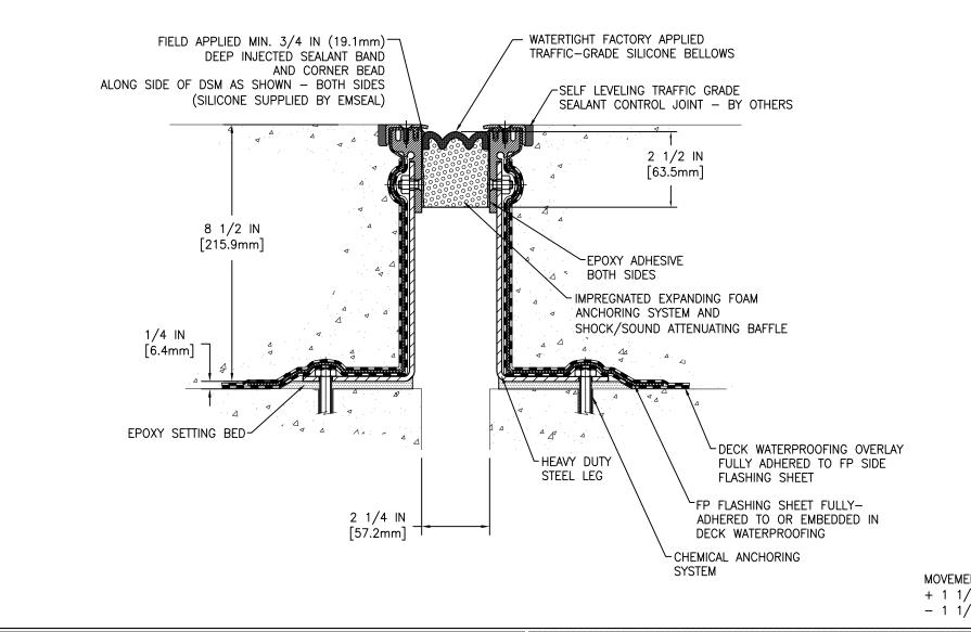
MOVEMENT: ±50% + 1 1/8 IN (29mm) - 1 1/8 IN (29mm)
