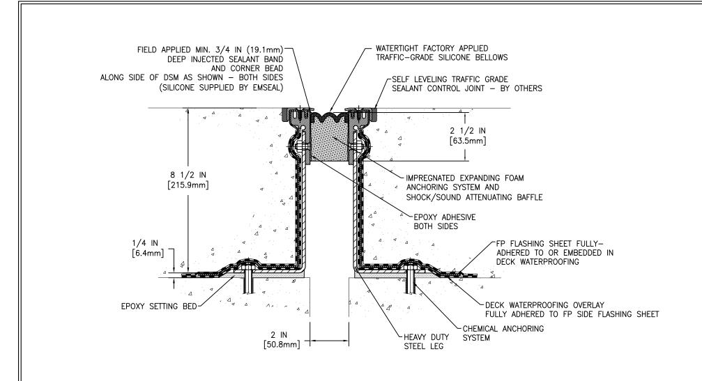
MOVEMENT: ±50% + 1 IN (25mm) - 1 IN (25mm)
