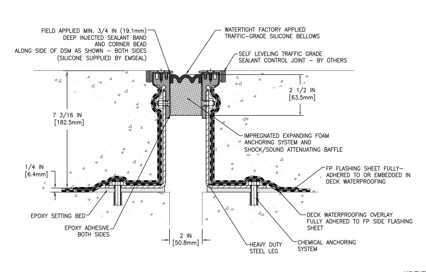
MOVEMENT: ±50% + 1 IN (25mm) - 1 IN (25mm)
