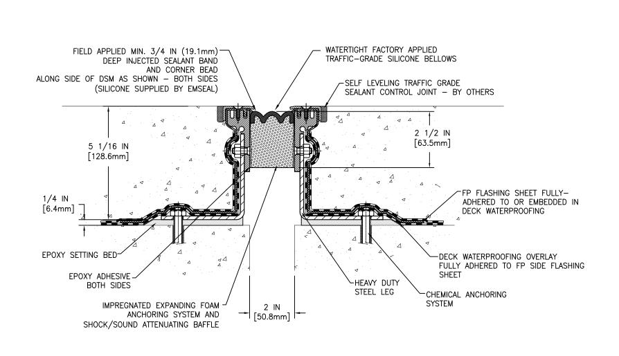
MOVEMENT: ±50% + 1 IN (25mm) - 1 IN (25mm)
