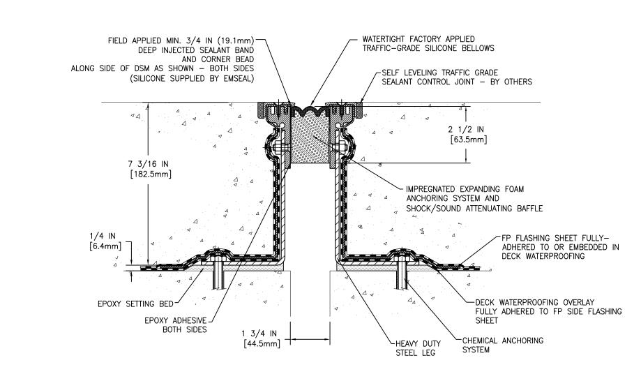
MOVEMENT: ±50% + 7/8 IN (22mm) - 7/8 IN (22mm)
