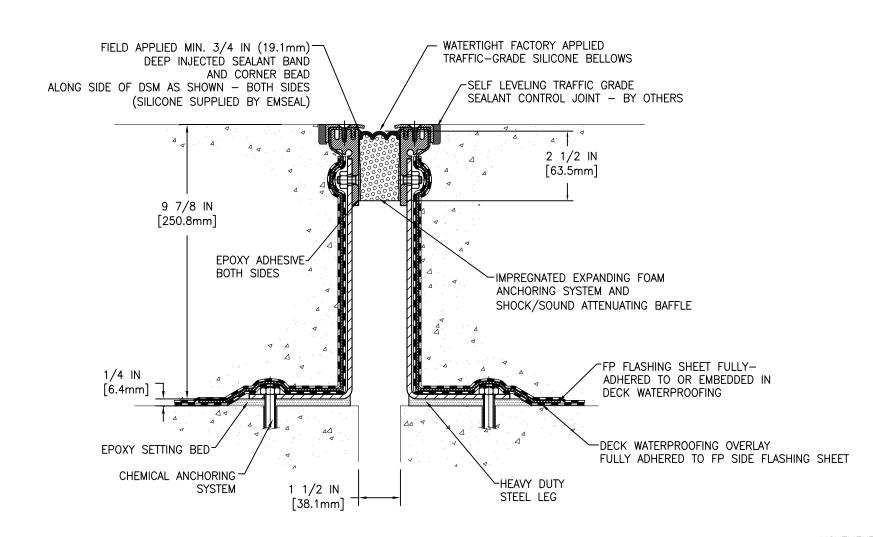
MOVEMENT: ±50% + 3/4 IN (19mm) - 3/4 IN (19mm)
