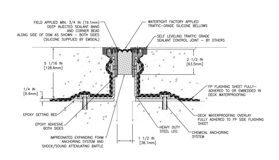
MOVEMENT: ±50% + 3/4 IN (19mm) - 3/4 IN (19mm)
