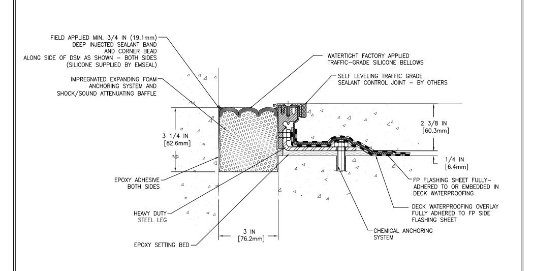
MOVEMENT: ±50% + 1 1/2 IN (38mm) - 1 1/2 IN (38mm)
