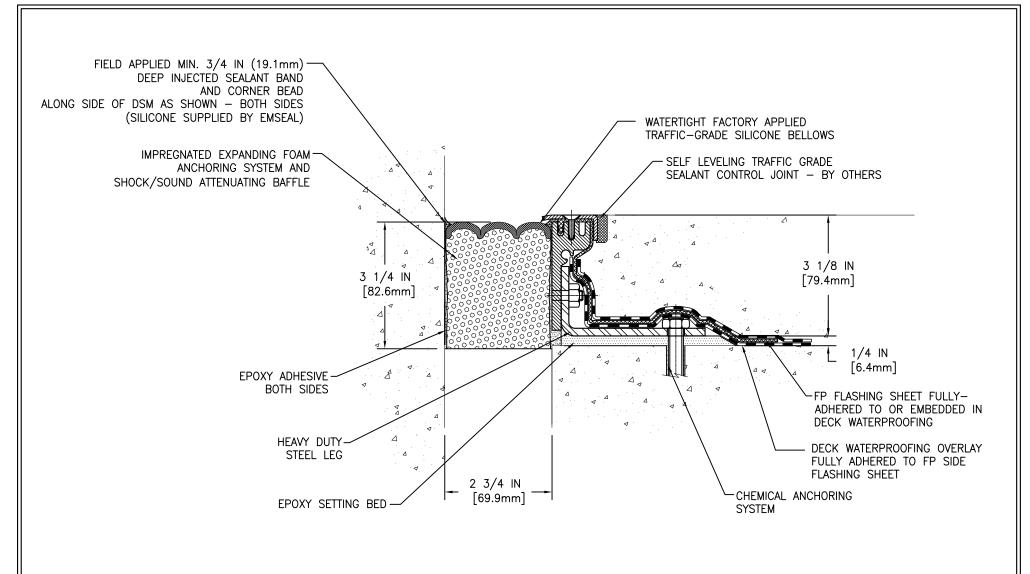
MOVEMENT: 50% + 1 3/8 IN (35mm) - 1 3/8 IN (35mm)
