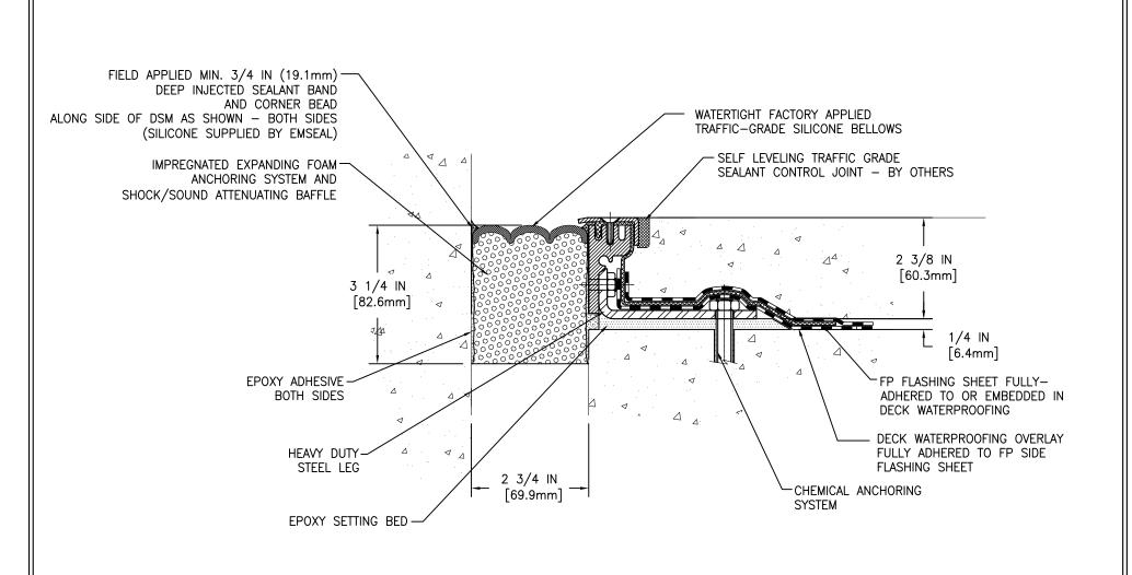
MOVEMENT: 50% + 1 3/8 IN (35mm) - 1 3/8 IN (35mm)
