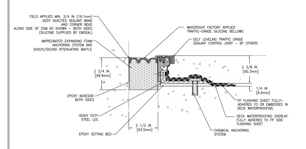
MOVEMENT: ±50% + 1 1/4 IN (32mm) - 1 1/4 IN (32mm)
