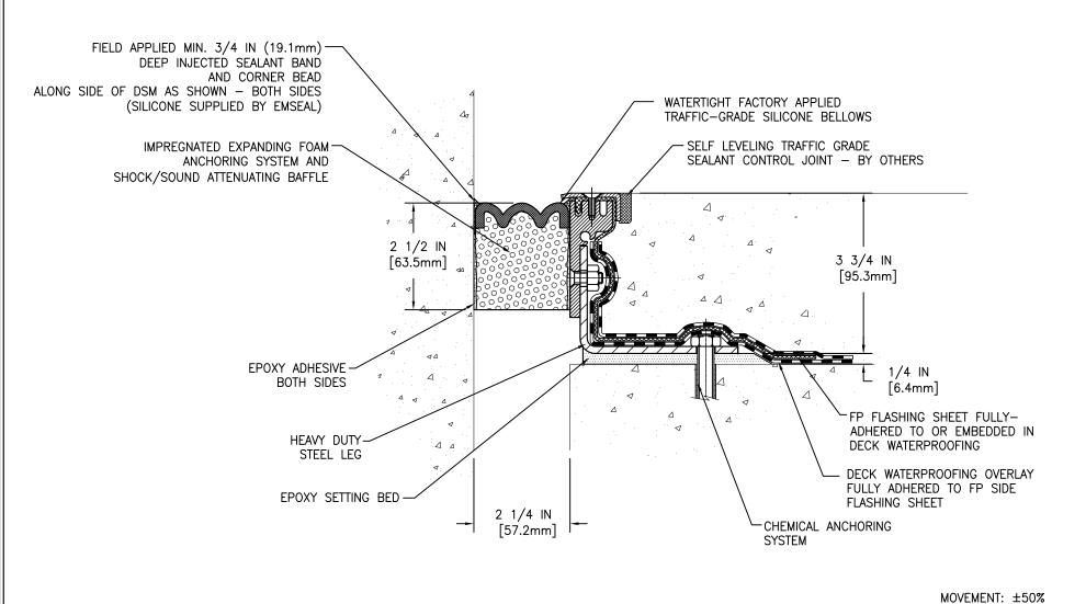
MOVEMENT: ±50% + 1 1/8 IN (29mm) - 1 1/8 IN (29mm)
