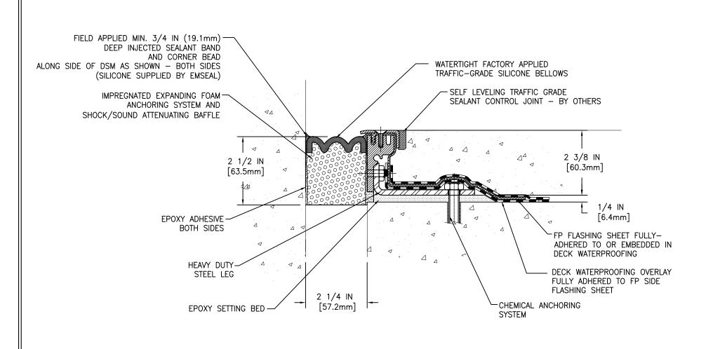
MOVEMENT: ±50% + 1 1/8 IN (29mm) - 1 1/8 IN (29mm)
