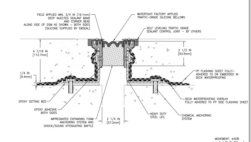
MOVEMENT: ±50% + 1 1/8 IN (29mm) - 1 1/8 IN (29mm)
