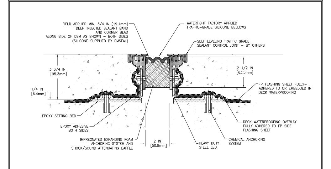
MOVEMENT: ±50% + 1 IN (25mm) - 1 IN (25mm)
