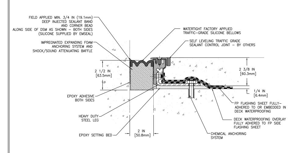
MOVEMENT: ±50% + 1 IN (25mm) - 1 IN (25mm)
