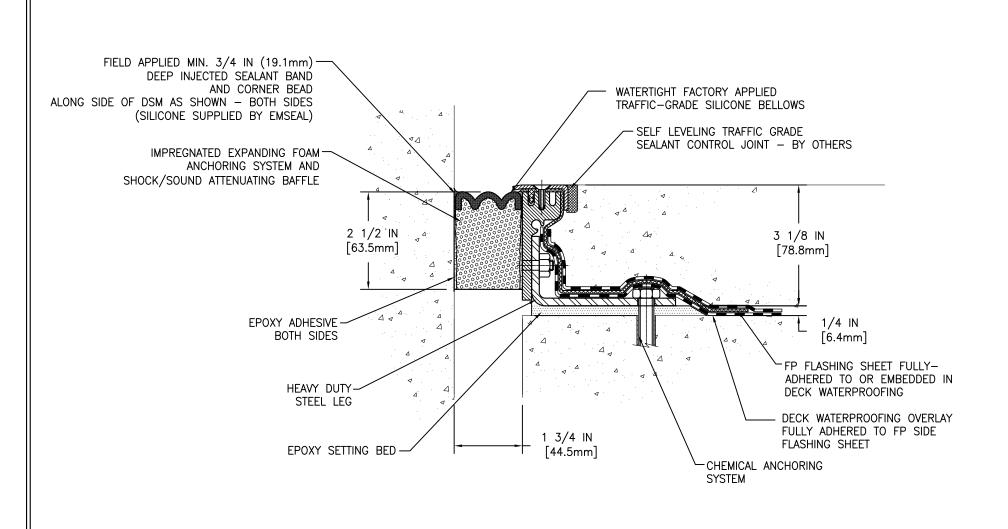
MOVEMENT: ±50% + 7/8 IN (22mm) - 7/8 IN (22mm)
