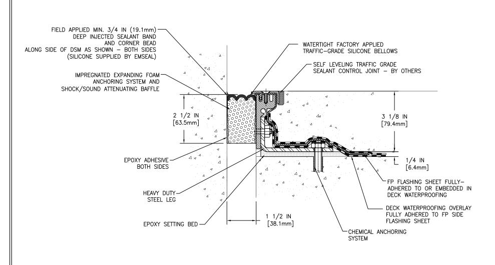
MOVEMENT: ±50% + 3/4 IN (19mm) - 3/4 IN (19mm)
